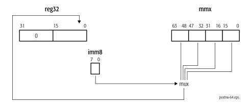
Table 1-1. Immediate-Byte Operand Encoding for 64-Bit PEXTRW
