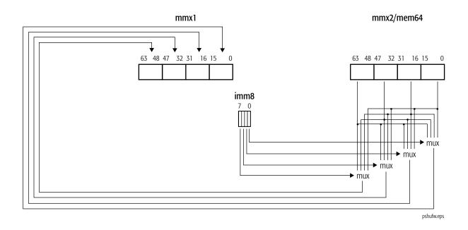
Table 1-20. Immediate-Byte Operand Encoding for PSHUFW
