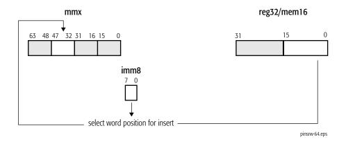
Table 1-19. Immediate-Byte Operand Encoding for 64-Bit PINSRW
