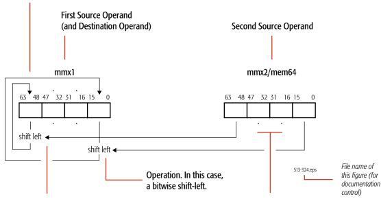
Arrowheads coming *from* a source operand indicate that the source operand provides a *control function*. In this case, the second source operand specifies the *number* of bits to shift, and the first source operand specifies the *data* to be shifted.
